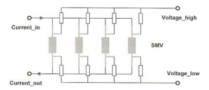
It is always possible to switch four-terminal resistors in parallel by connecting the current terminals. The question is were to measure the voltage. If all series resistances formed by the copper connections to the resisistors (i.e. PC-board tracks) are equal than all resistors see the same current and in this case it is not important one which resistor the voltage is measured.
